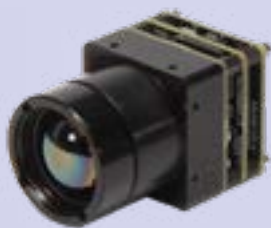
Core camera with 13.6mm lens (32° HFOV)
