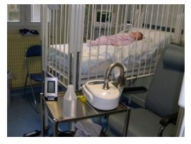
The Coriolis  $\mu$  air sampler has been already used in French hospitals for monitoring winter epidemics of bronchiolitis & gastro-enteritis. It has been shown that the Coriolis µ air sampler coupled with PCR detection method is able to detect virus in patient narrow environment and thus prevent from epidemic dissemination. The Coriolis  $\mu$  can be used for:
