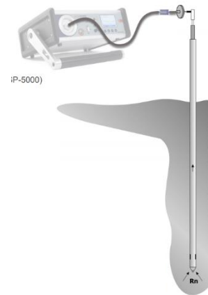
Soil Gas probe
